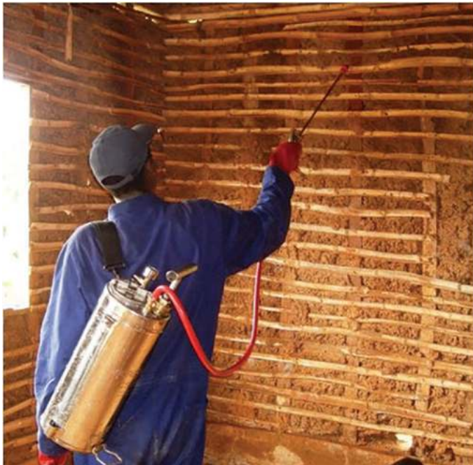
Fig. 8.2. Indoor residual spraying with a hand-operated sprayer equipped with a control flow valve and the operator wearing PPE
